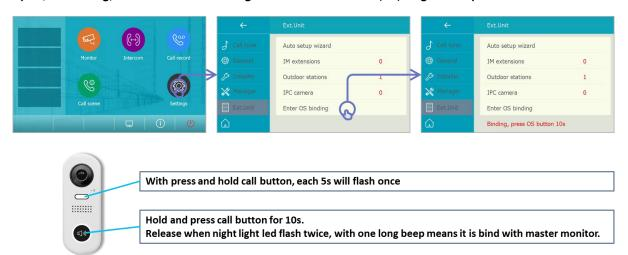
On the master monitor need to be called, tap "Settings" -> "ExternalUnit" -> "Enter OS binding", and when "Binding, please press OS button 10s" shows on the bottom,
