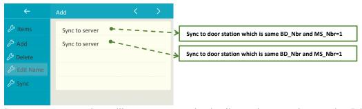
**Sync to server**, monitor will generate a monitoring list, and sync to door station DS1. **Sync from server**, monitor will get IP camera list storage in door station DS1.
